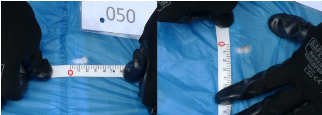
Photo 11: A Ripped Hole (1 cm X 2 cm) on the Paragliding Canopy
